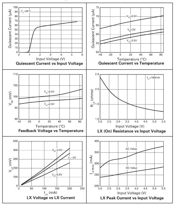
TYPICAL CHARACTERISTICS (For typical application circuit at  $V_{\rm IN}{=}3V$  and TA=25  $^\circ\rm C$  unless otherwise stated)
