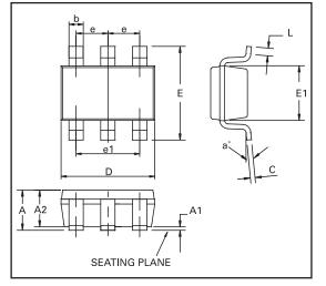
Controlling dimensions are in millimeters. Approximate conversions are given in inches
